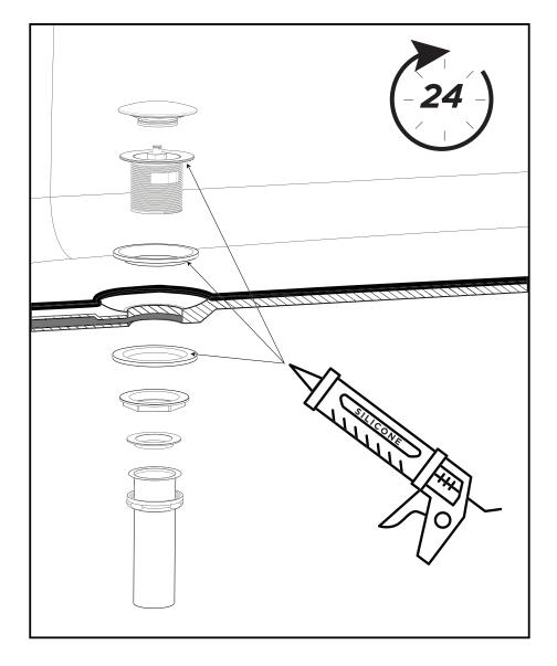
Elevate the bath by blocking under the legs and water test the drain and overflow. Check for water leaks and ensure proper drainage.
