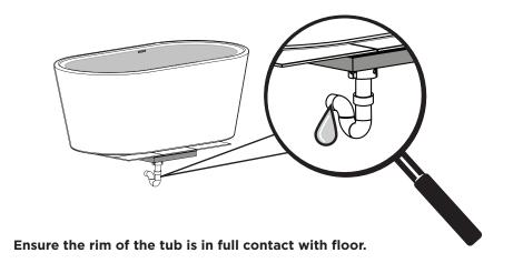
Step 7 Seal around the base of the tub with silicone sealant
