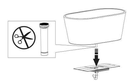
Ensure the drain pipe is properly connected, and verify the bath is level. Fill the bathtub and do a drainage test to ensure the bath drains properly. Check for and correct any water leaks.
