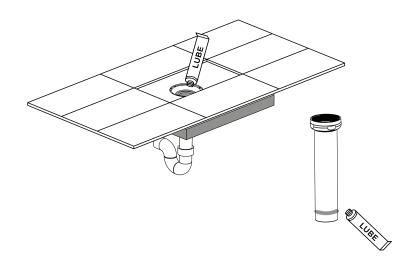
**Step 5**Place the bath onto the EZ Drain assembly
