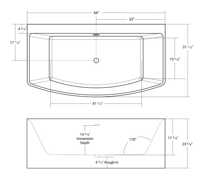
If the Semi-freestanding tub is going against any wall, the tub to be installed with the supplied tiling flange.
